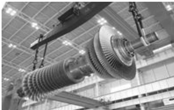
Figure 2 J-series MHI gas turbine capable of operating at TIT = 1,600°C.
