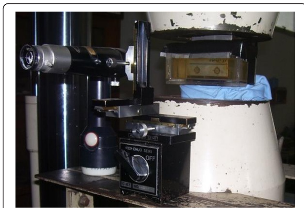
Figure 4 The corrosion chamber used in the corrosion fatigue test.
