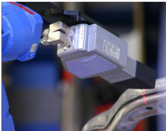
Fig. 5 Three-dimensional weld seam inspection by VIRO WSI (VITRONIC 2010)
