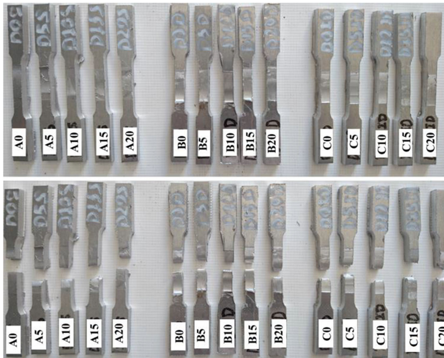
Fig. 12 The fracture location of the studied samples
