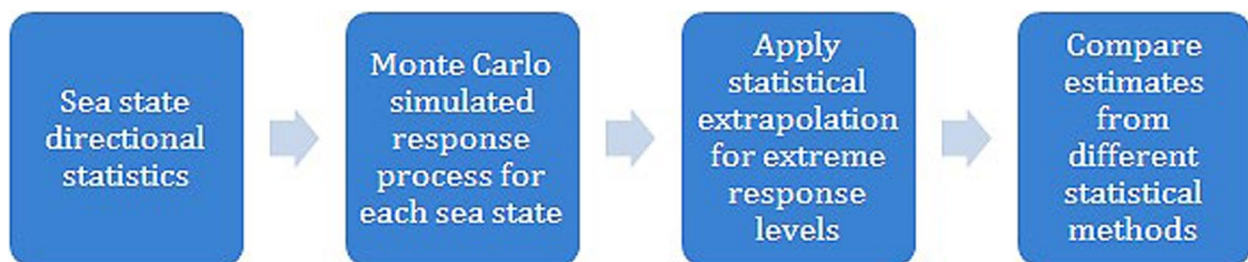
Fig. 2 Long-term MC-based reliability flowchart
