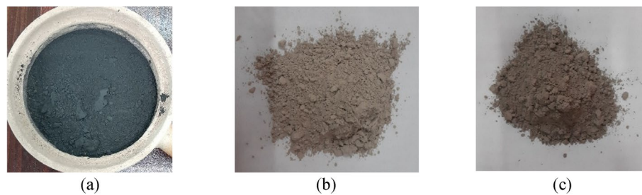
Fig. 1 The black color of ground POFA (a) changes to gray color micro POFA (b), and (c) is the 50k nano POFA
