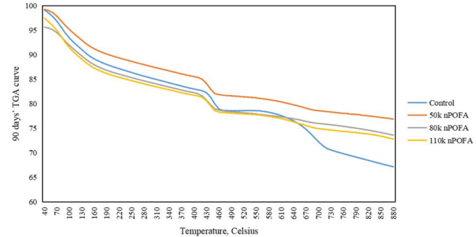
(c) Summary of the TGA curve of cement paste that either controls or contains three types of nano POFA at the 90-day curing age.
