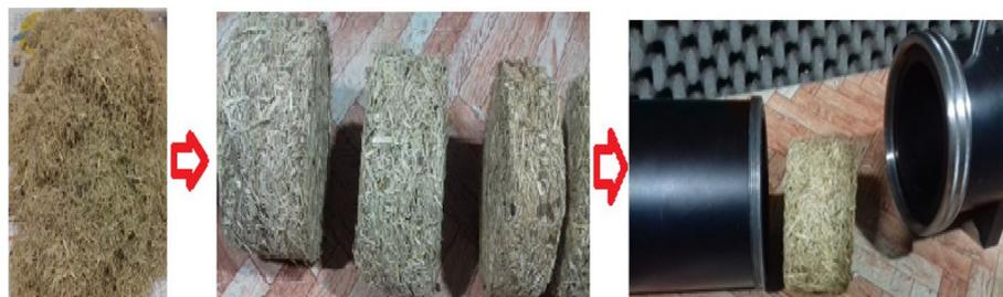
**Fig. 2** Making of sugarcane fiber composite and measurement of its sound absorption coefficient by tube impedance device (Beheshti et al. 2022)
