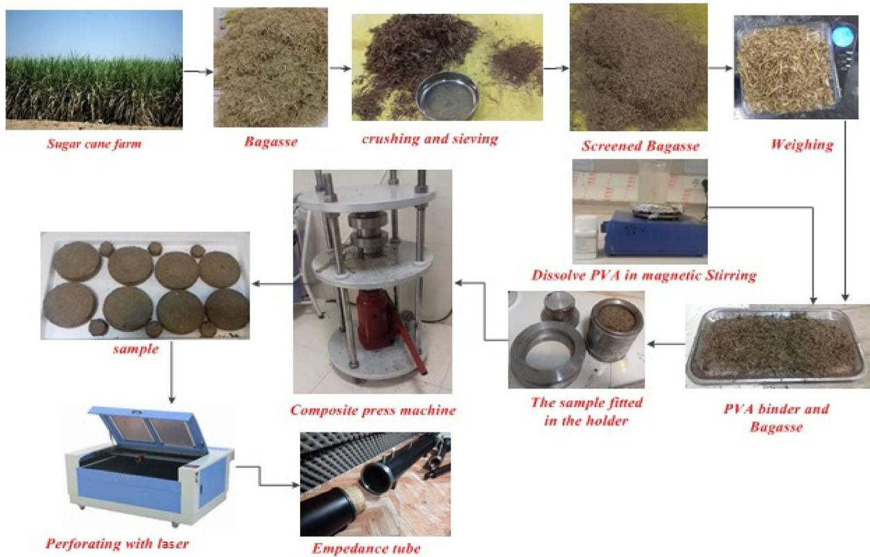
**Fig. 3** The steps of making natural MPP using bagasse
